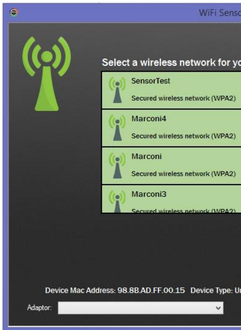
On the Wireless Network selection screen, click on the green antenna symbol on the top left of the window. This will cause a dropdown box to appear on the bottom left. Select the network adaptor which corresponds to the same network as the WiFi Sensors. Then continue the setup as normal.
