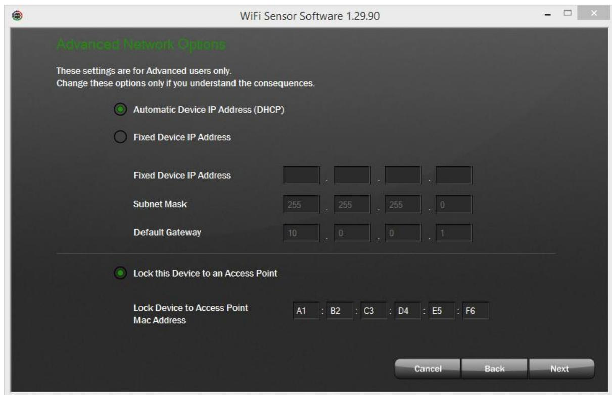
Enter the MAC Address of the access point you want to lock the sensor to.
