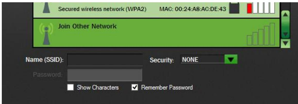
The SSID may contain invalid characters. The wifi sensors are unable to handle certain special characters such as spaces or commas in the SSID or trailing spaces at the end. You may need to change the SSID of the network. This also applies to passwords.
